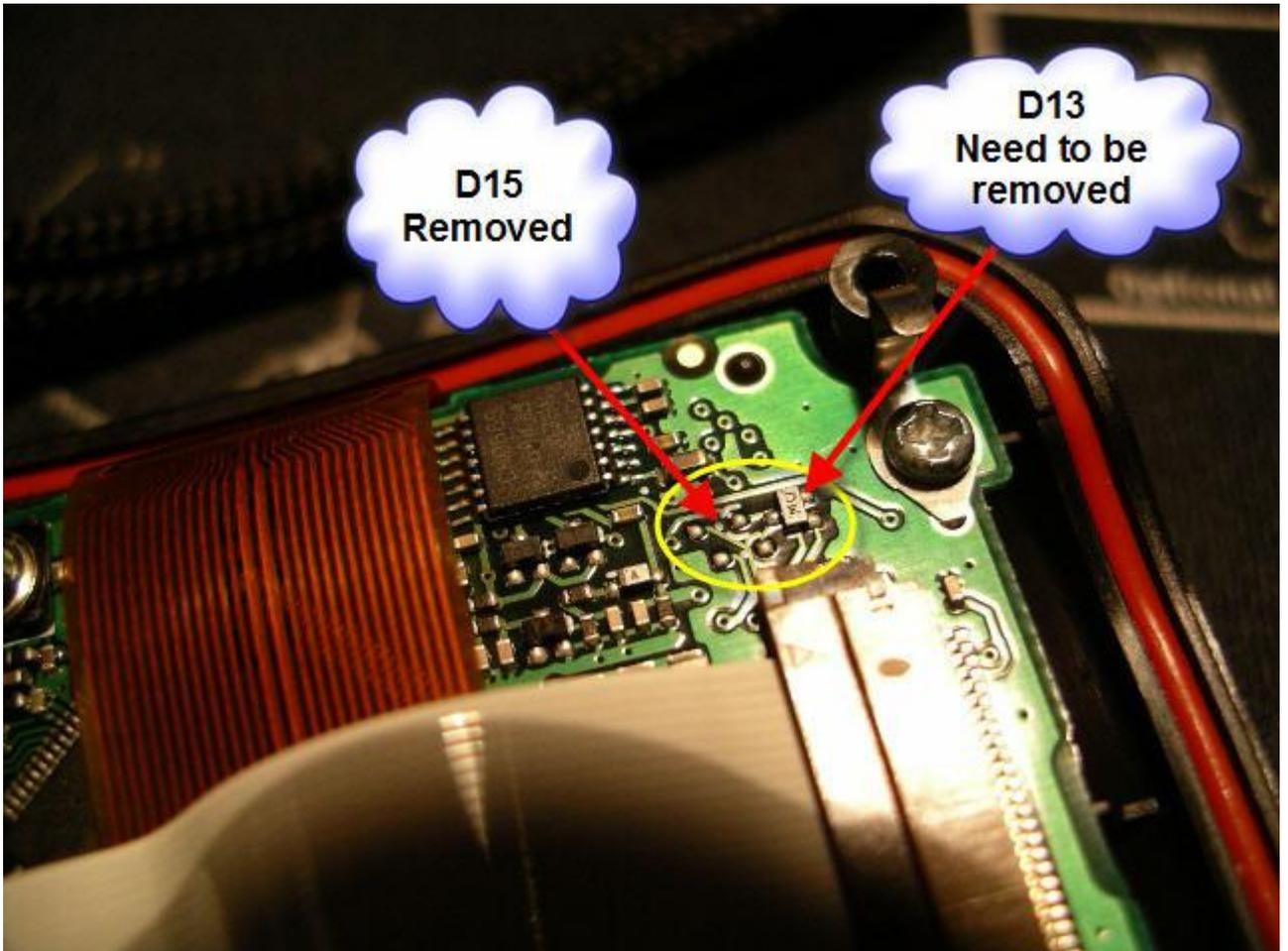
The "TX/RX Frequency of IC91/IC-E91" modification works!
